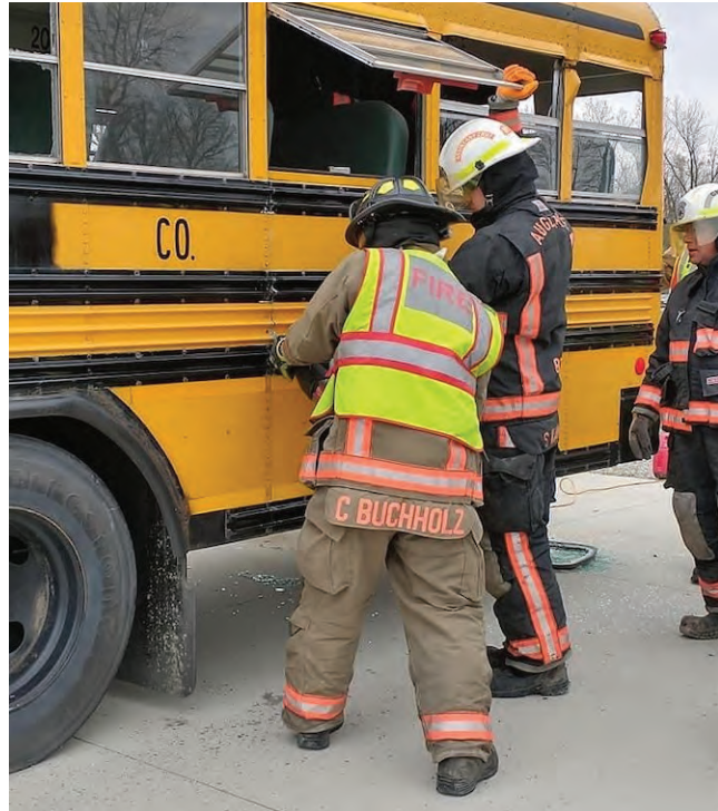
Pictured here are firefighter making access to the side of the bus with battery operated power tools and saws.
