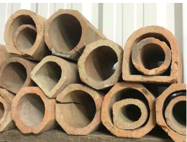
The John Paulding Historical Society has a collection of clay drainage tiles that illustrate the evolution of design. Among them are flat-bottomed horseshoe, round with flat base, hexagonal, octagonal and the more familiar round.
