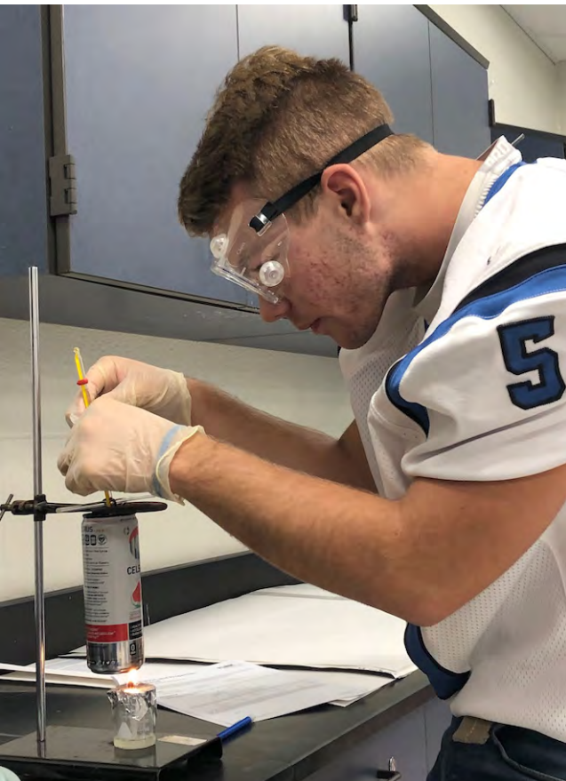
Pictured: Junior Dylan Hines measures the temperature of the water in the can as the biodiesel in the small beaker heats it from below.
