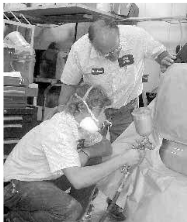
Vantage Auto Body instructor John Kenueke watches closely as senior Jonathan Young from Lincolnview applies paint to a fender using an HVLP gravity spray gun.
