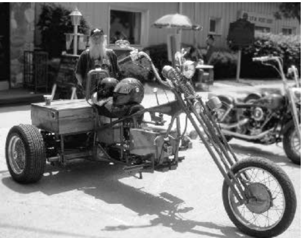
A Handmade motorcycle. Michael Garberson, of Grover Hill decided he wanted to build his own cycle. He calls it a "trike". It has a '69 Volkswagen motor, a Harley frame, Springer front end. He has a wooden battery box that holds the battery and the wiring and his shifter is a glass doorknob out of a house. He built it 16 years ago and it took him 1 year to build. He is now in the process of building one for someone else.
