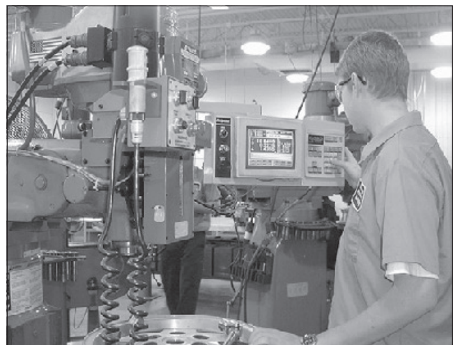
Evan Gordon, a junior in the Vantage Precision Machining Technology program from Wayne Trace, programs the CNC mill to engrave an aluminum truck rim.
